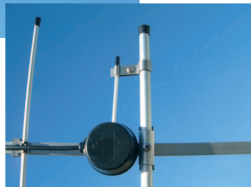
● Fig. 2: The gamma match bar is covered in ptfе making a capacitive contact through the clamp to the driven element.
